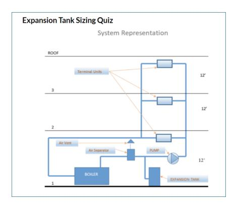
The sizing and selection of expansion and compression tanks is straightforward when the engineer has the proper information. Today, we list the seven things you need before sizing a tank and offer a sample problem for you to try while reading.
